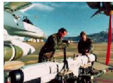
Self-defense jamming pods, such as the ALQ-184, use various deception techniques.
